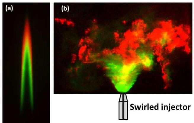
Figure 1: (a) Overlay of LII (red) and LIF-PAH (green) on CH<sub>4</sub>/air laminar diffusion flame at atmospheric pressure. (b) Overlay of LII (red) and LIF-PAH (green) obtained from Jet A-1/air combustion on MICADO test rig at  $p = 7.14$  bar.
